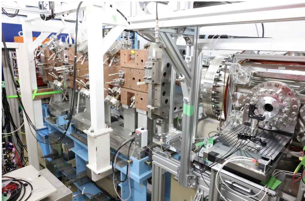
Figure 2 Experimental set up for muon cooling and acceleration at the J-PARC Materials and Life Science Experimental Facility (MLF). A positive muon beam enters from the right side, is cooled in the muon cooling chamber on the right and is accelerated in the radio-frequency acceleration cavity on the left. The accelerated muon beam is measured by a diagnostics system at the exit of the acceleration cavity.
