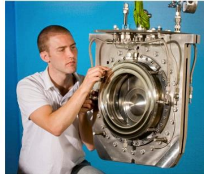
Figure 1 : (Left) The “beam window” is a thin wall separating the accelerator from the target station. High intensity proton beams, accelerated towards the target, are repeatedly injected through the beam window. (Right) The beam window at the J-PARC neutrino experimental facility, fabricated from high-strength titanium alloy Ti-6Al-4V (Copyright: STFC RAL).
