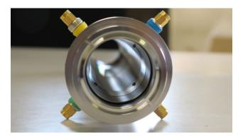
Fig.1. Wideband beam monitor with four rod antennas located at every 90°.
