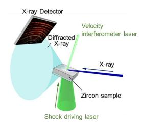
Fig. 1: Configuration of the laser shock experiment.
