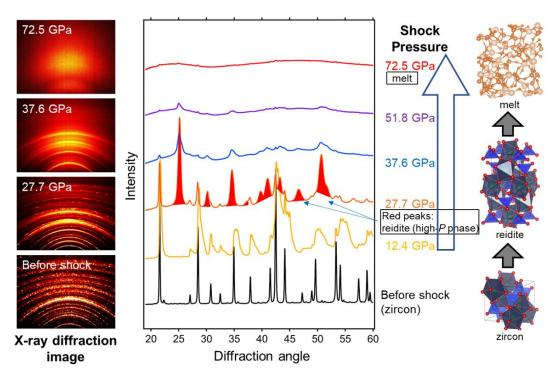
Fig. 2: X-ray diffraction data for a laser-induced shock.
