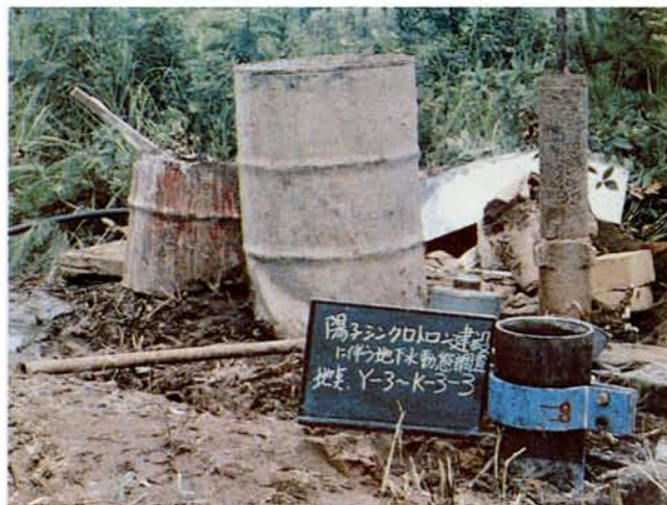
加速器建設予定地にて地下水位調査(43年、筑波) Underground water level is surveyed at the site planned for the accelerator construction (1968, Tsukuba).
