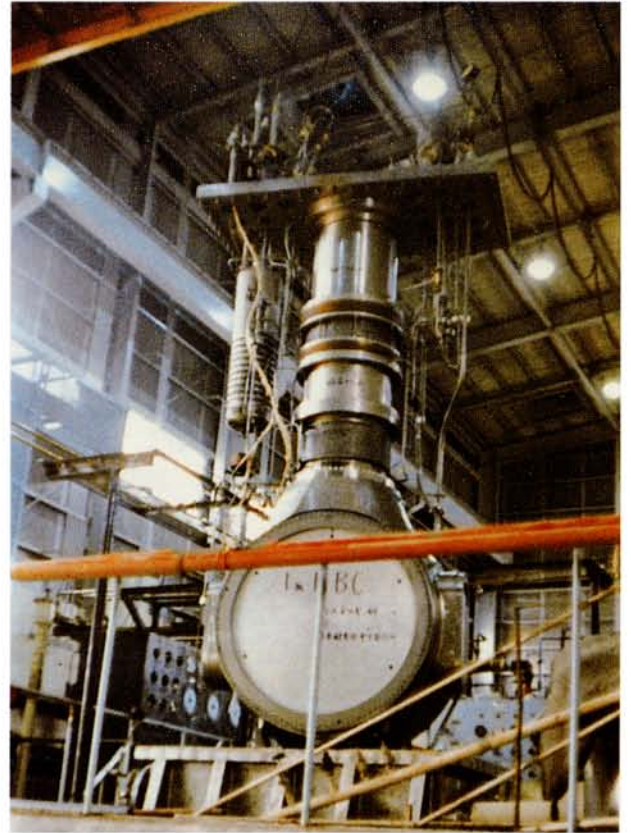
1 m水素泡箱 The one-meter hydrogen bubble chamber.
