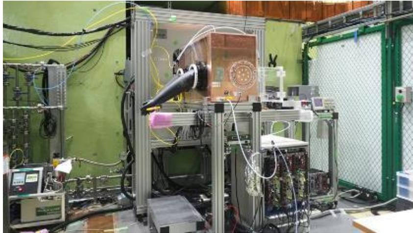
Figure 3: The custom-made experiment setup developed to avoid the samples from being contaminated by the Earth's atmosphere. The interior is filled with helium gas, and the chamber is lined with pure copper to minimize background noise. (Credit: KEK IMSS)
