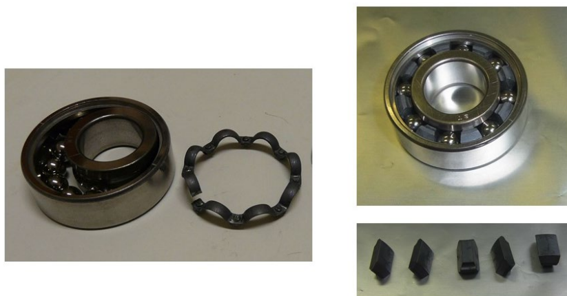
Figure 2: Conventional bearings using solid lubricants are coated with molybdenum disulfide or silver on the balls, an outer ring, an inner ring, and a ball separator (left); J-PARC uses a bearing with lumps of tungsten disulfide (bottom right) inserted between the balls (top right).
