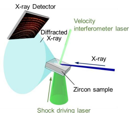
Fig. 1: Configuration of the laser shock experiment.
