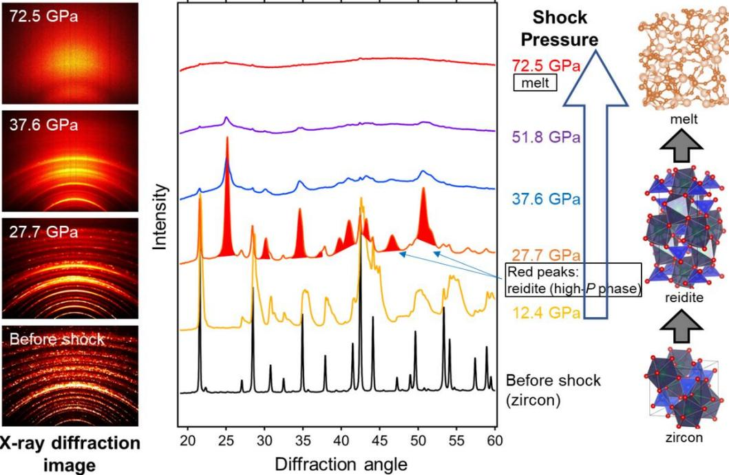
Fig. 2: X-ray diffraction data for a laser-induced shock.
