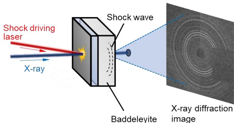
Figure 2. Experimental configuration of time-resolved X-ray diffraction measurement under laser-induced shock conditions.
