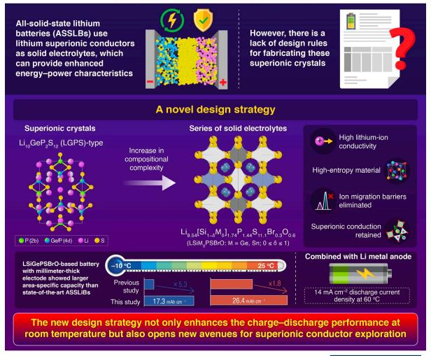
A lithium superionic conductor for millimeter-thick battery electrode
